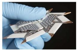
A revolutionary battery that uses virtually any droplets of water to work has been developed. It is foldable, disposable and low in cost. Aimed to provide people in developing nations with a portable source of electrical power. Also, find out more about this battery in <u>Sciencedirect</u>.
