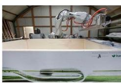
Presenting 3D Builder! It's a robot that can transport itself around a building site to print stone or concrete buildings. It can also recycle its own products by forming buildings out of waste concrete or stone. Also, see the 3D builder at work in this video.
