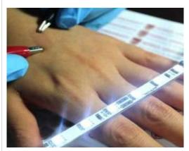
Researchers from the University of Illinois and Korea University produced a bendable, stretchable film that is extremely thin. The film consists of looping nanofibres and it will be used in wearable electronic devices. In addition, you can find out more about this film at Wiley.
