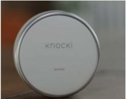
Knocki is a smart gadget that can instantly make any surface smart. Sticking to a surface like a table or a door, Knocki is able to interpret a pattern of knocks or taps into commands, such as brewing your coffee from bed, adjusting room temperature, or anything that can be programmed over Wi-Fi.
