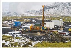
In Iceland, researchers discovered a new method to fight climate change by locking up the greenhouse gas without leakage. Carbon Dioxide was pumped into deep underground and amazingly it transformed into new carbonate minerals that may stay there forever. Additionally, get more details about this process in Science.
